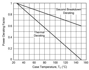
There are two limitations on the power handling ability of a transistor: average junction temperature and second breakdown. Safe operating area curves indicate  $l_{\text{c}}$  -  $V_{\text{CE}}$  limits of the transistor that must be observed for reliable operation; i.e., the transistor must not be subjected to greater dissipation than the curves indicate.
